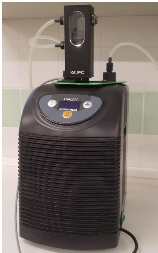
Fig. 8 Water cooling unit AC-700.
