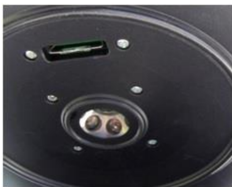
Fig. 4 Ring of excitation LEDs in optical part of MU.
