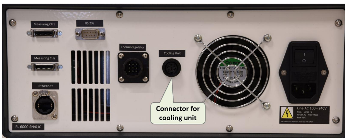
Fig. 15 Connector for Nitrogen cooling unit.
