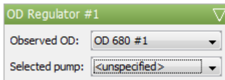
Fig. 35 OD regulator control panel for MC
