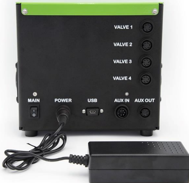
Fig. 3 Power cord connection to the PP 600.
