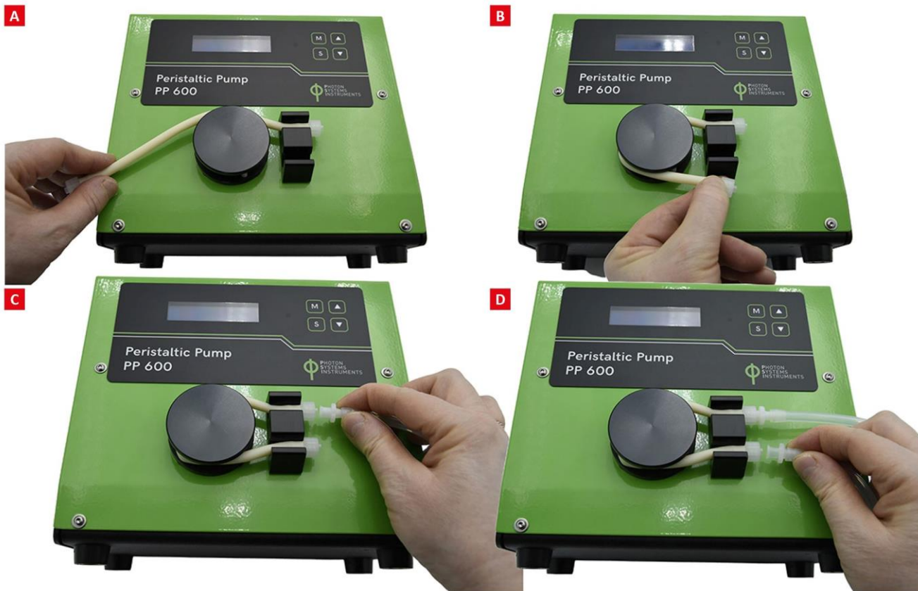
Fig. 4 Assembly of the Peristaltic Pump.
