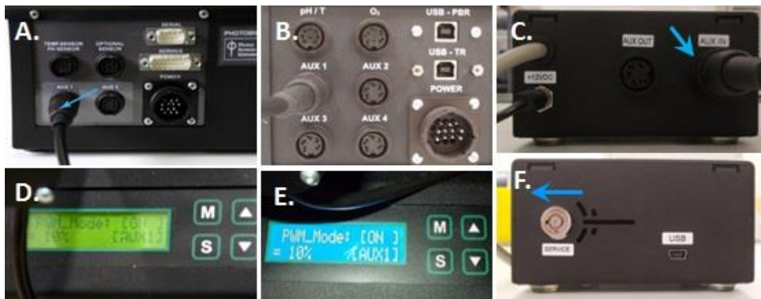
Fig. 35 A, B, C) Attaching of the communication cable to the “AUX 1” and “AUX IN” (A – FMT150.1 version; B, C – FMT150.2 version). D, E) Manual Stirrer control via the PWM_Mode on the front panel of PBR (D – FMT150.1 version; E – FMT150.2 version). F) Horizontal position of the service button.
