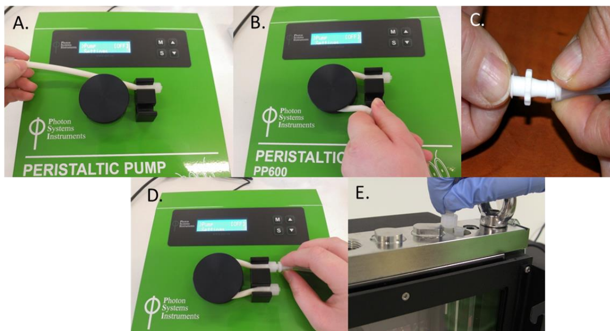
Fig. 47 Assembly of the peristaltic pump. A, B) Short tube is attached around the rotor wheel to the peristaltic pump. C, D) Adapter is attached to the silicone tubing and connected with the tubing of the peristaltic pump. E) Tubing from the peristaltic pump is connected with the cultivation vessel.
