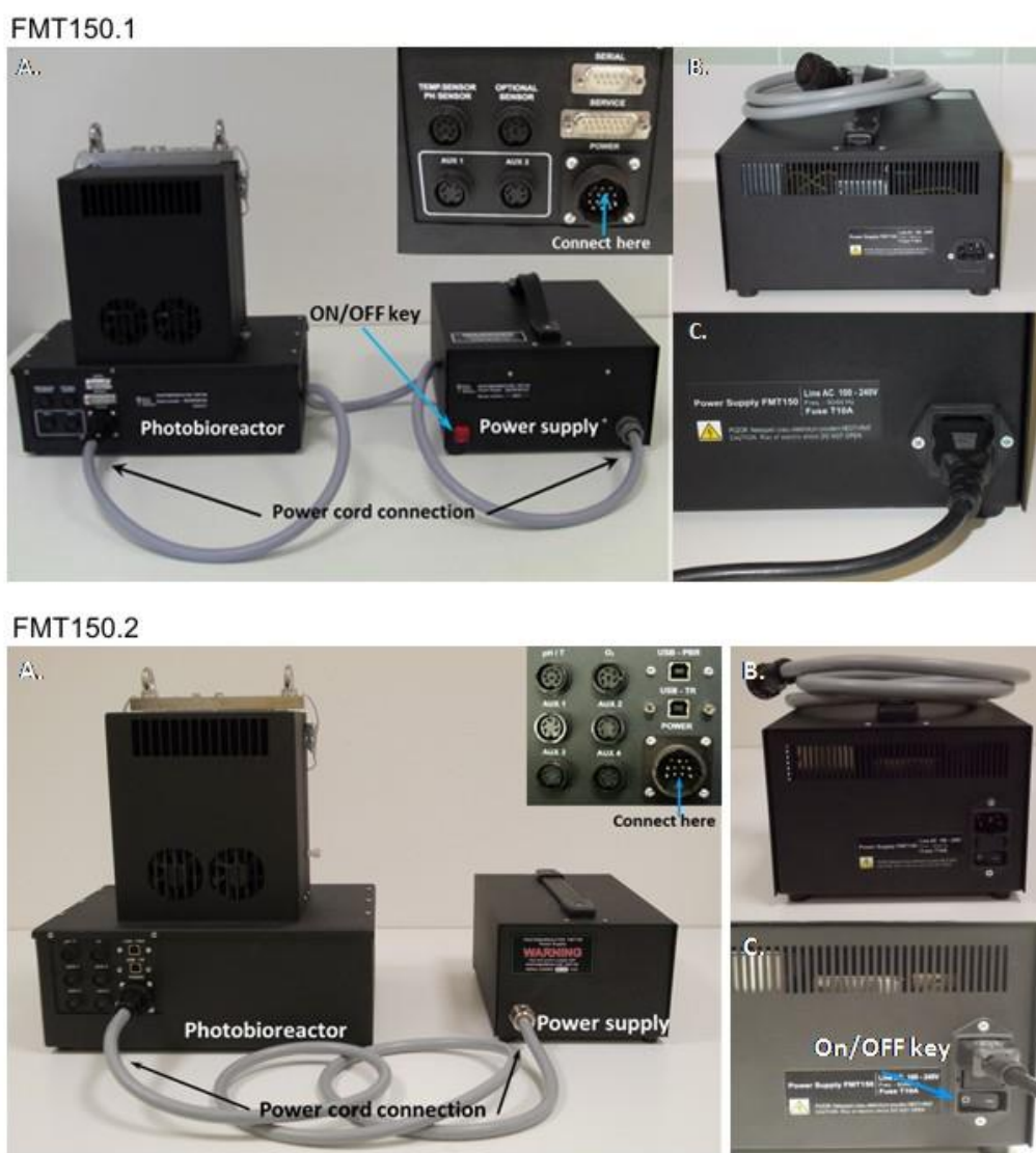
Fig. 11 Connection of the Photobioreactor and the power supply. A) Top right panel shows detail view of the back panel of the Photobioreactor. B) C) AC power cord connection to the electrical outlet.
