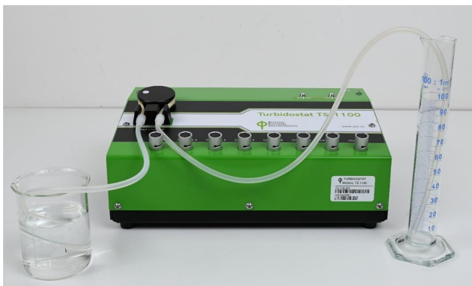
Fig. 6 Set up of Turbidostat module for calibration.
