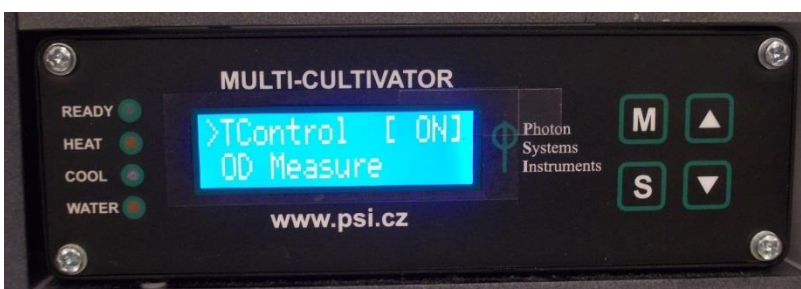
Fig. 10 Display of the MC 1000-OD control unit when Cooling Unit AC-710 is operating.
