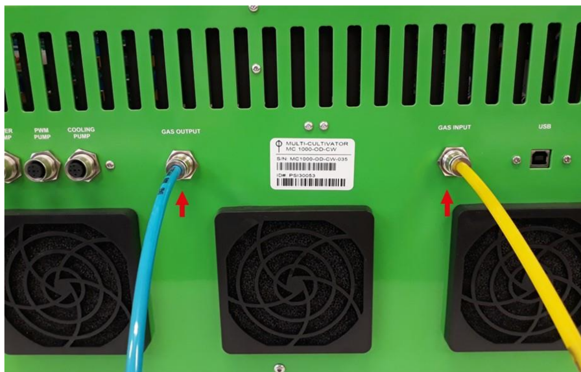
Fig. 11 Rear panel of MC 1000-OD version with gas/air mixing module.
