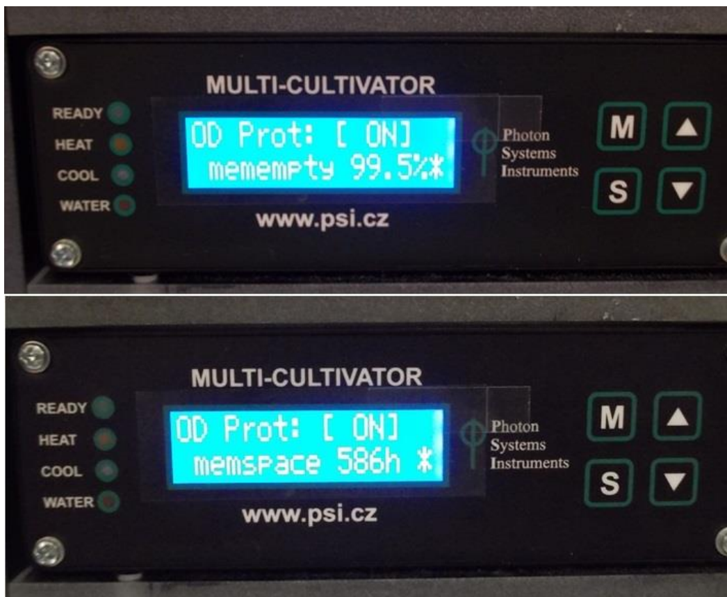
Fig. 23 Control unit display with remaining memory space in % and in hours is shown.
