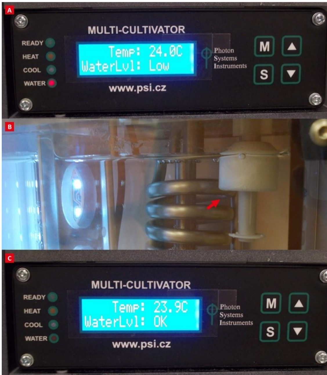
Fig. 19 Water level controller.
