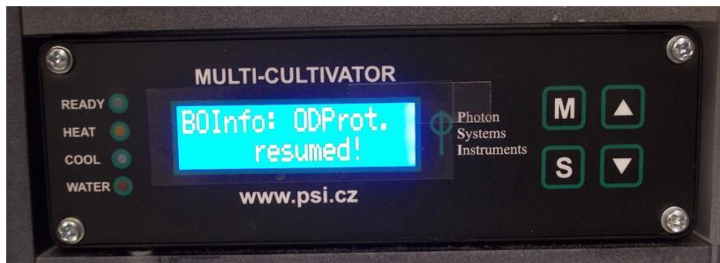
Fig. 29 Control unit display after OD protocol was resumed following MC 1000-OD power outage.
