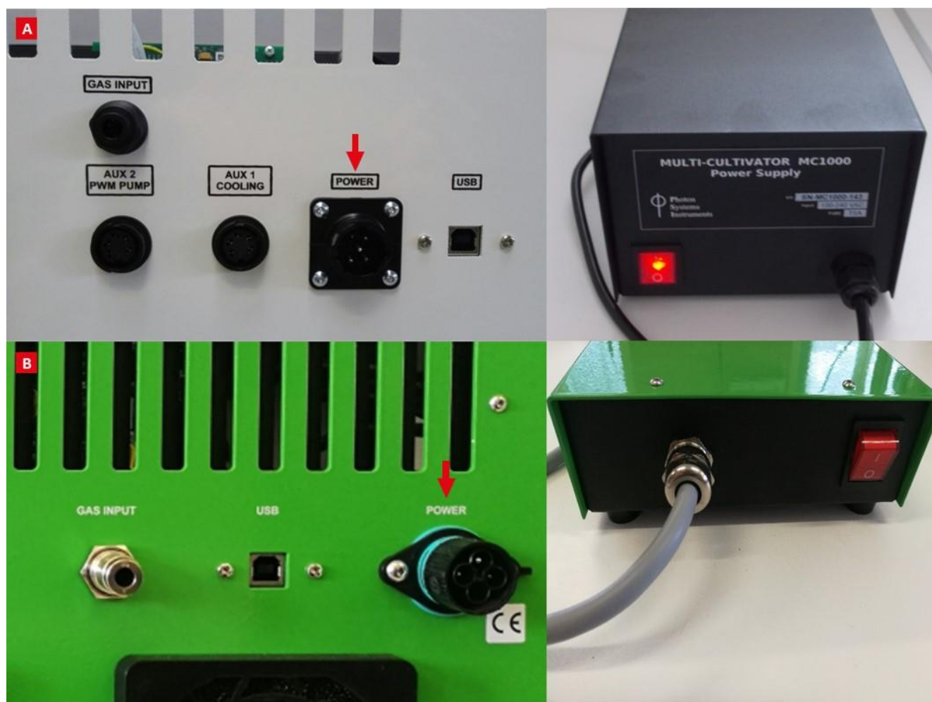
Fig. 6 Rear panel of MC 1000-OD with POWER connector and Power supply device.
