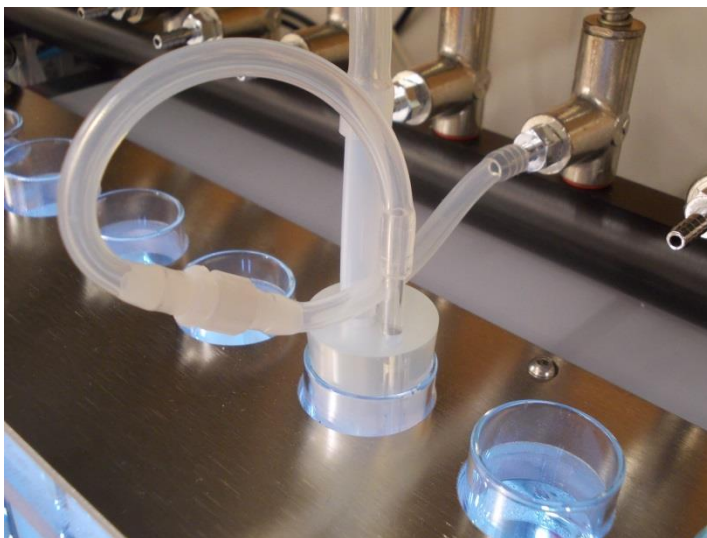
Fig. 21 Connection of the cultivation tube to the main gas dispenser tube.
