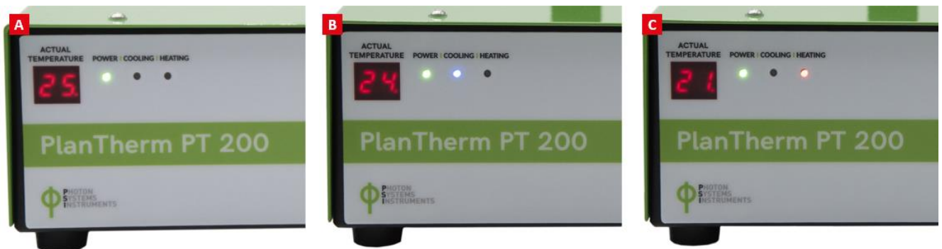
Fig. 4 LED signaling: A) green LED for switched on device, B) blue LED for cooling, and C) red LED for heating.
