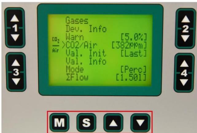
Fig. 12 Setting Screen – main menu and keys for operating the menu.
