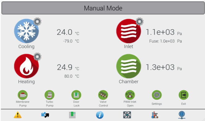
Figure 31: Red Inlet icon_ set fuse limit has been exceeded
