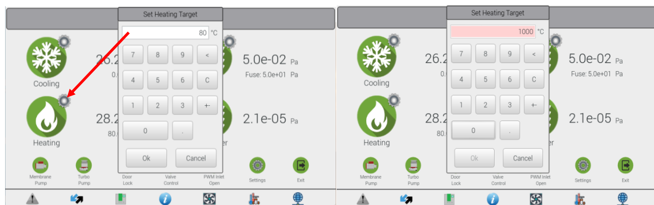
Figure 28: Setting of heating temperature, the wrong value of set temperature
