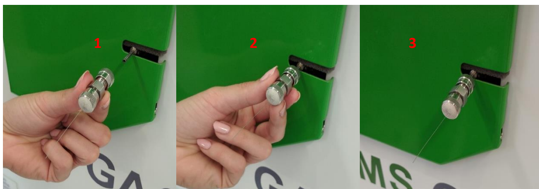
Figure 48: Procedure of needle input connection to MS GAS-100
