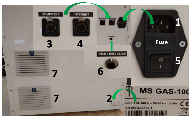
Figure 40: MS GAS-100 rear panel: 1) Power supply connector 2) MS GAS-100 label with serial number. 3) Ethernet connector 4) Firmware communication connector 5) ON/OFF switch 6) Input for Venting Gas 7) Fans
