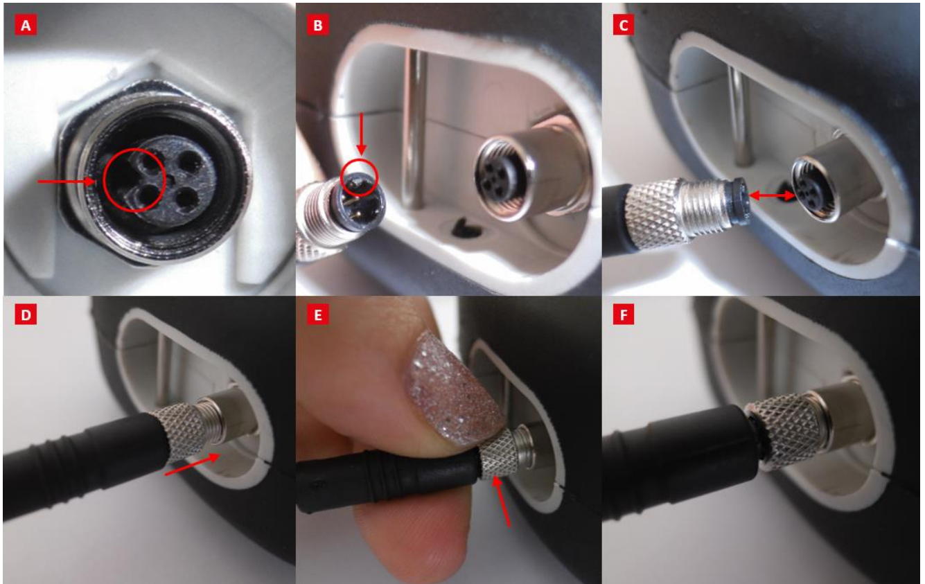
Fig. 12 How to connect PolyPen-Aqua with PC.
