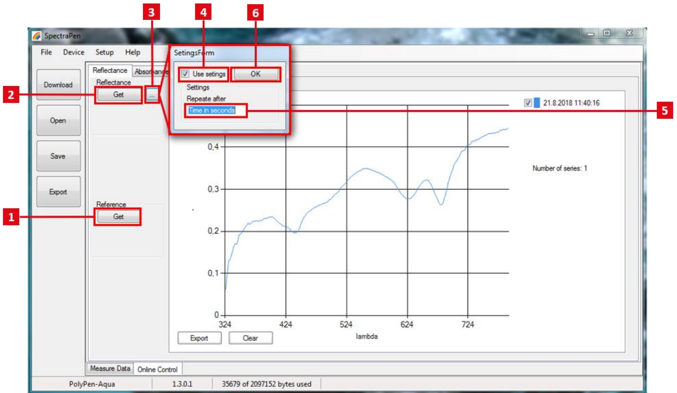
Fig. 36 Setting of reflectance or absorbance measurements in online control.
