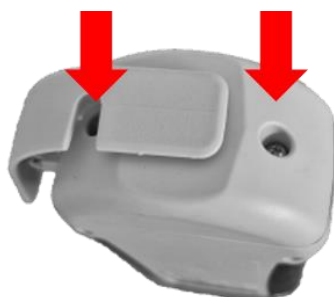
Fig. 4 Optical head can be removed for the purpose of cleaning. The part is attached to the device by 2 screws (red arrows)
