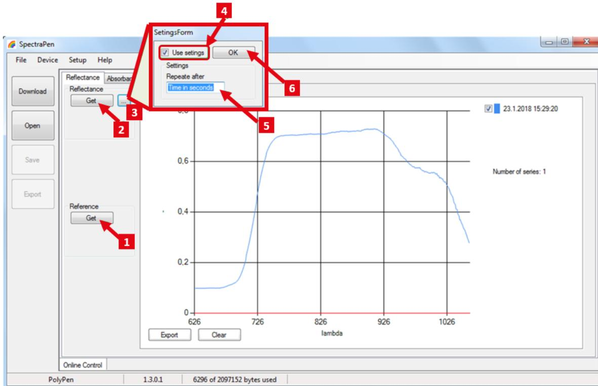
Fig. 36 Setting of reflectance or absorbance measurements in online control.
