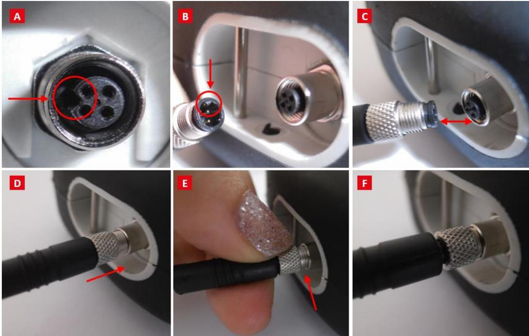
Fig. 12 How to connect PolyPen with PC.
