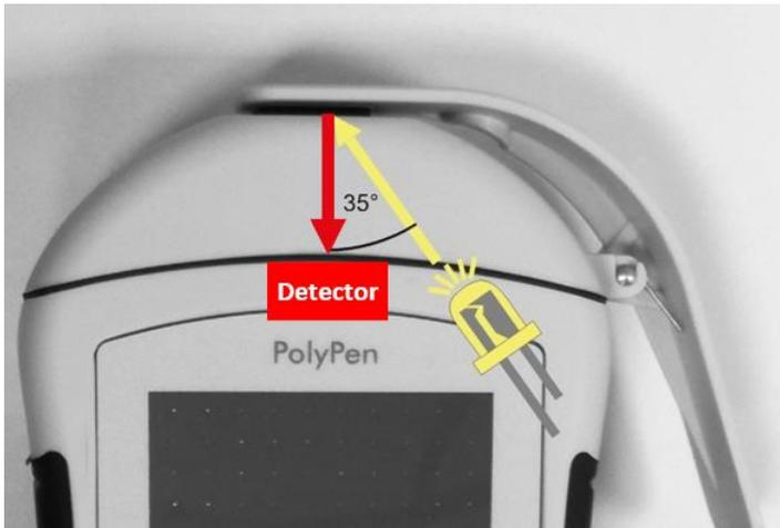
Fig. 2 Schema of reflectance measurement.
