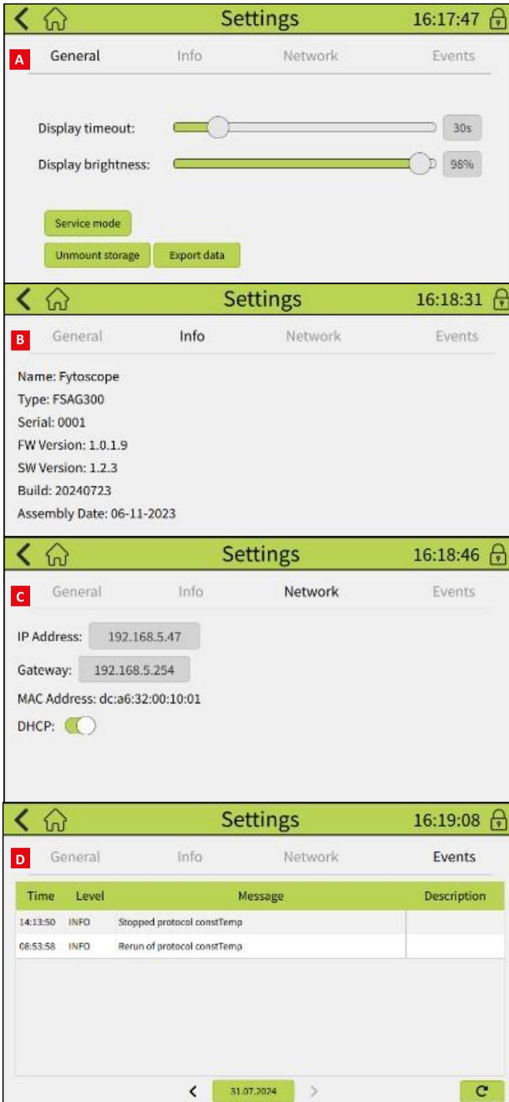
**[A]** The **General** tab offers setting of **Display timeout**, which sets the duration of inactivity after which the GUI automatically returns to the **Overview screen** (see Chapter 4.1). Another function is the configuration of **Display brightness**.
