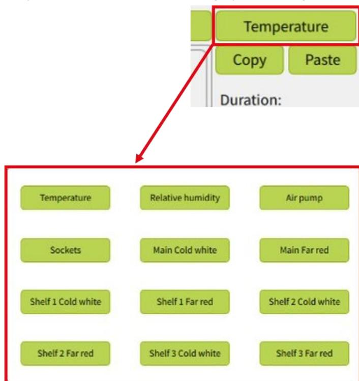
(Fig. 18 [1]). For each phase, set the duration and the desired value (temperature in °C, light intensity in %, activity of the pump, and devices plugged into sockets as ON/OFF).
