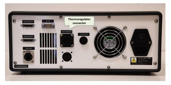
Fig. 3 Rear side of FL 6000 control unit.
