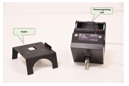
Fig. 1 Thermoregulator components.
