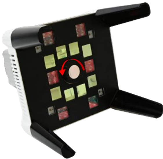
Fig. 18 Emission filters changing
