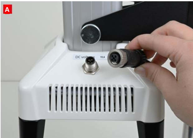
Fig. 7 Flat Handy FluorCam power source connection
