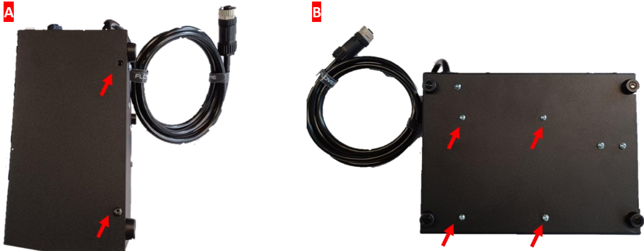
Fig. 30 Unscrew the two screws on each side of the battery box and open it, then remove the four screws securing the battery holder at the bottom of the battery pack.
