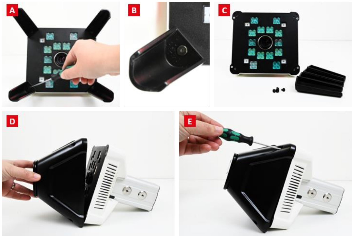
Fig. 7 Removal of the Flat Handy FluorCam's legs and installation of the Leaf clip
