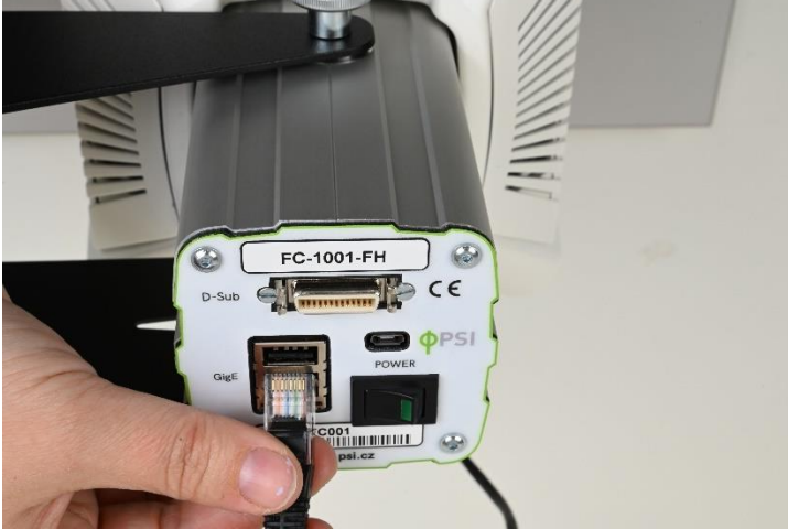
Fig. 6 Flat Handy FluorCam connection with PC through Ethernet cable
