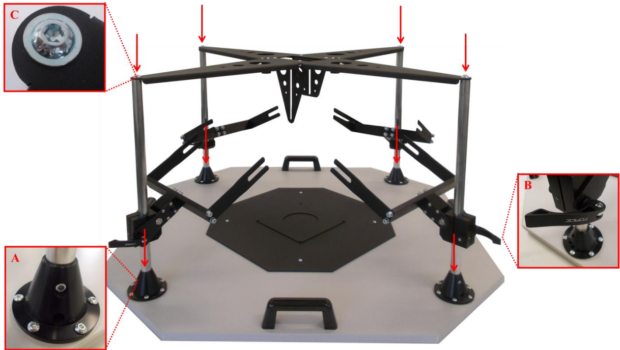
FIGURE 18. Open FluorCam stand assembly
