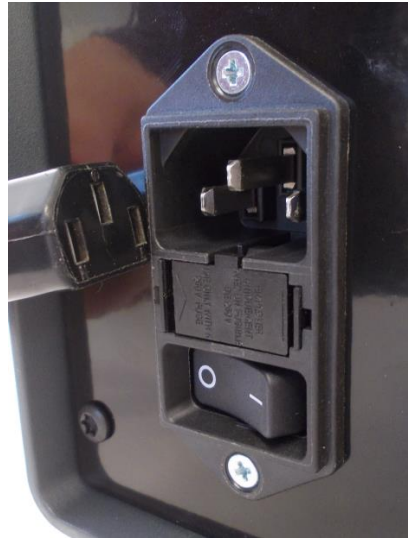
FIGURE 23. Backside of the Control unit - power supply cable connection
