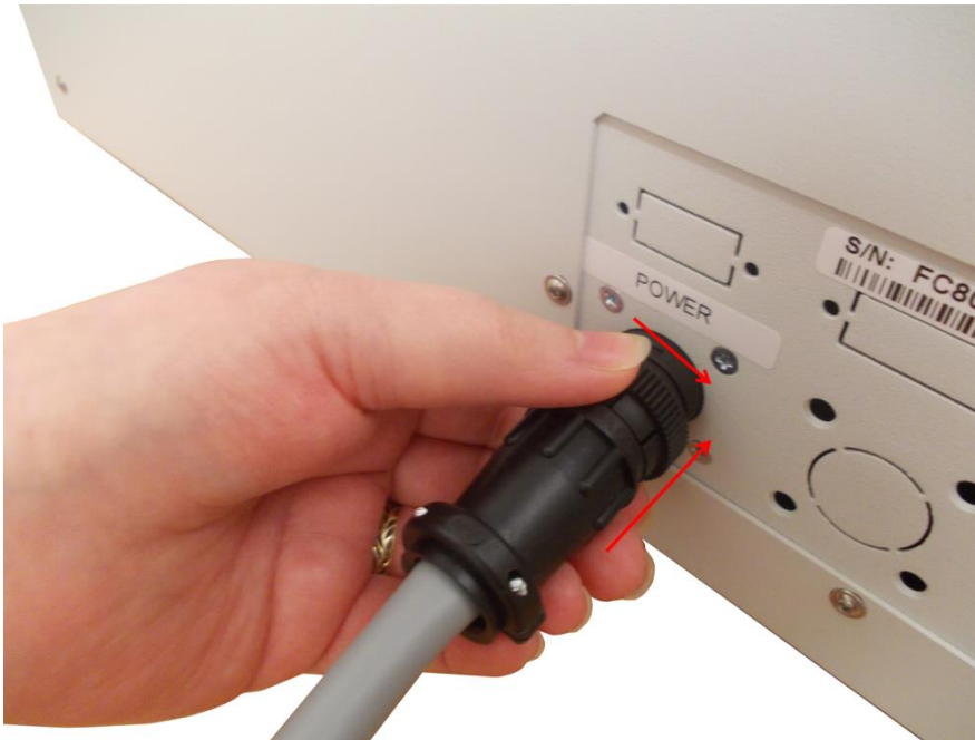
FIGURE 14. Power cable connection
