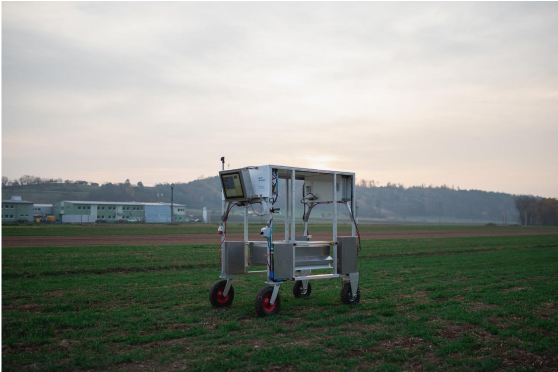
FIGURE 10. Rover FluorCam is a remarkably stable structure. Its large and solid wheels, which are motorized, allow easy movement in a terrain
