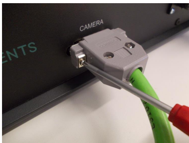
FIGURE 22. Camera connection with Control unit
