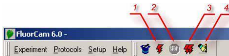
FIGURE 32. Top icon bar of the FluorCam software. (1) Trigger starting compilation of the protocol (if not done in the protocol window) and initiating execution of the experiment. (2) Stop interrupts execution of the experiment. The experiment can be re-started (but not resumed) after the stop is used. (3) Multiple trigger with automatic bar code reading and file assignment. (4) Manually activated bar code reader.
