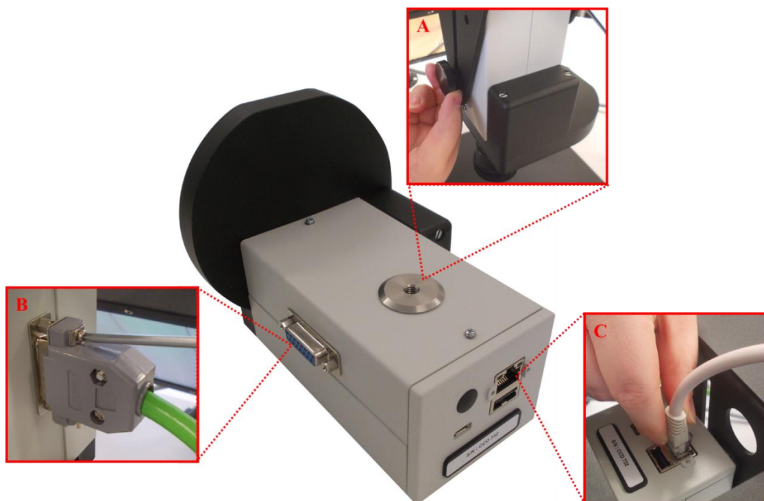
FIGURE 21. FluorCam camera with filter-wheel. A) Mounting of camera to the support brackets and tightening with the knob, B) Connecting camera with Control unit, C) Connecting camera with PC
