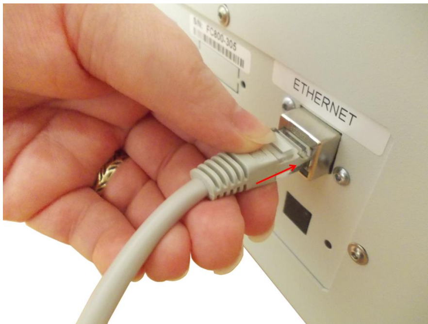
FIGURE 15. Ethernet cable connection
