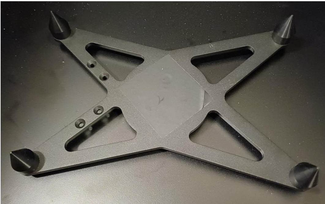
Fig. 5 Thorns for precise positioning of the tray with plants.
