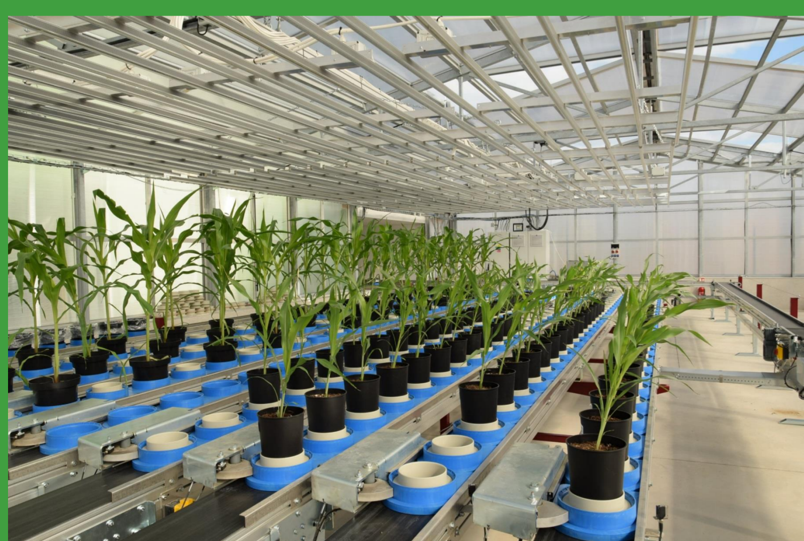
PlantScreen™ Modular System for automated phenotyping of 270 plants up to 1.5 m in height in greenhouse environment.
