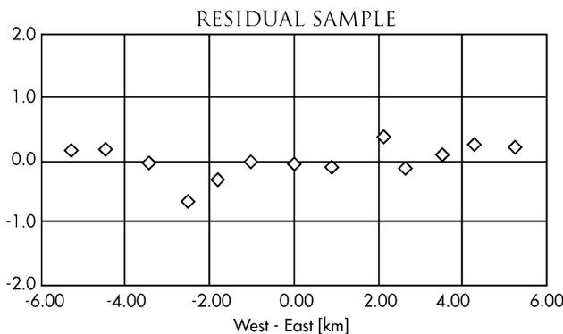
Fig. 10. Post-FAM-calibration residual errors over the southern test range displayed against the GCP layout; no significant systematic error pattern.
