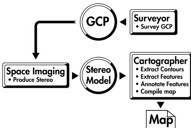
Fig. 14. Cartographic extraction from stereo images.
