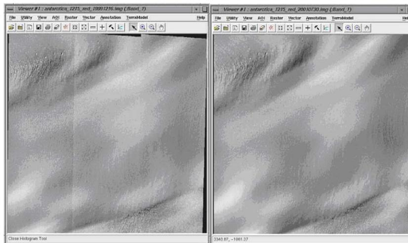
Fig. 5. Relative radiometric uniformity requirements demonstrated on Antarctic snowfield uniform scene. Left: Visible banding artifacts still visible after radiometric correction to better than 10 counts or 0.8%. Right: Radiometric uniformity is now better than 0.5% over the dynamic range of the detectors (Imagery<sup>®</sup> Space Imaging).
