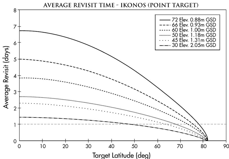
Fig. 1. Relationship between IKONOS revisit intervals, latitude, sensor elevation angles, and GSD.
