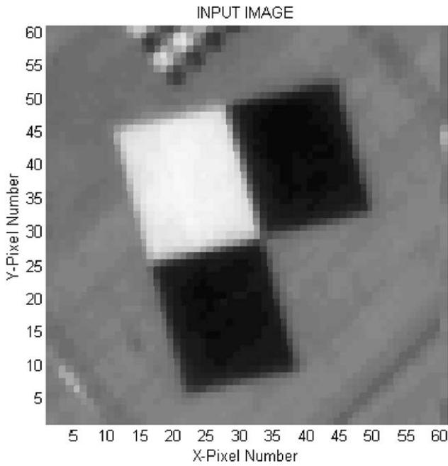
Fig. 3. IKONOS image of edge target used for modulation transfer function measurements (Imagery<sup>®</sup> Space Imaging).
