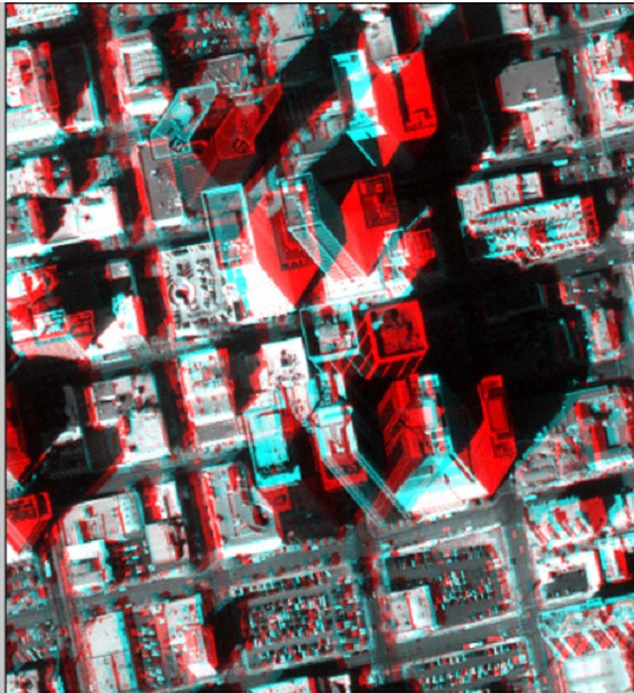
Fig. 16. Anaglyph visualization made from an IKONOS stereo pair (Imagery<sup>®</sup> Space Imaging).
