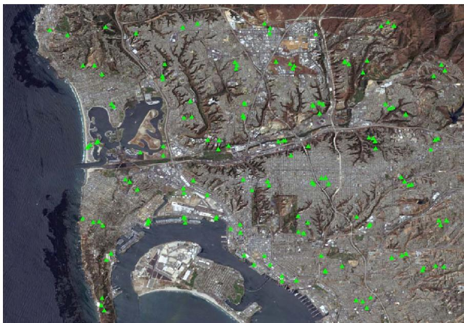
Fig. 8. IKONOS geometric accuracy testing range over San Diego consisting of 140 ground control points over a  $22 \times 22$ -km area (Imagery<sup>®</sup> Space Imaging).
