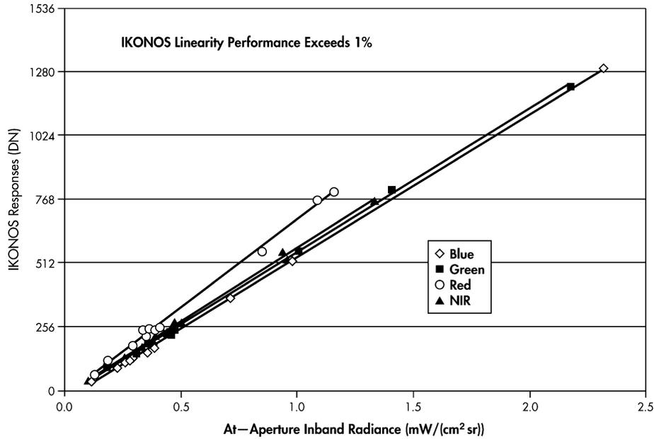
Fig. 6. IKONOS radiometric linearity.
