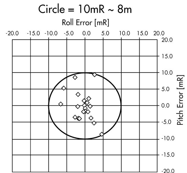
Fig. 11. Error distribution after corrections applied to improve interlock angle calibration.
