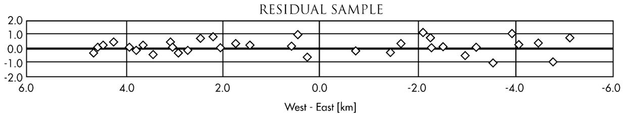
Fig. 9. Post-FAM-calibration residual errors over the Denver test range displayed against the GCP layout; no significant systematic error pattern.
