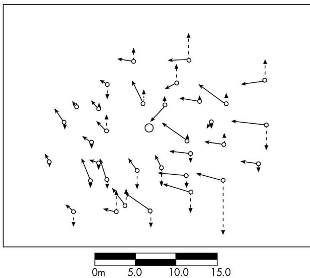
Fig. 12. Validation of FAM and interlock calibrations, and quantification of block adjustment accuracy: vertical and horizontal errors shown by dotted and solid arrows, respectively, for a case with a single GCP.
