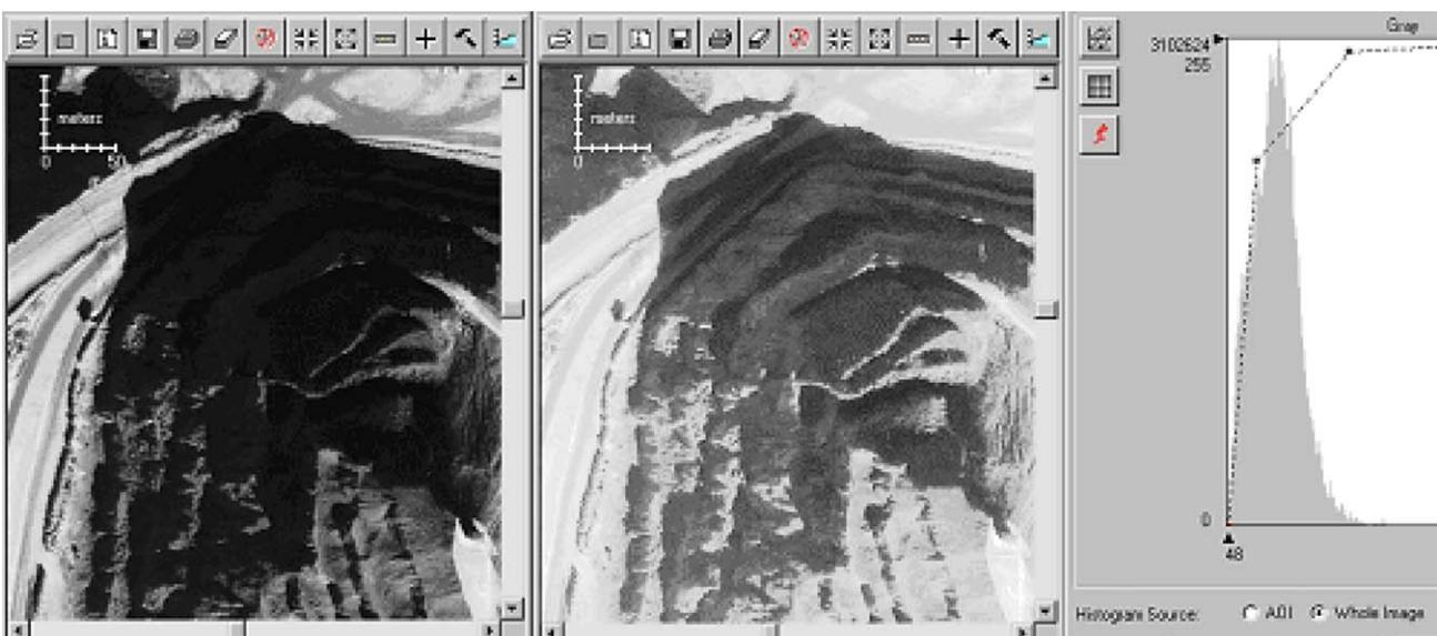
Fig. 13. Extracting detail from shadows in 11-bit imagery. Left: Image displayed with full radiometric range. Right: Same image stretched to show detail in shadows.
