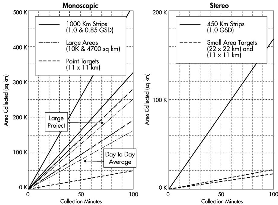
Fig. 2. Area collection rates for monoscopic and stereo images.
