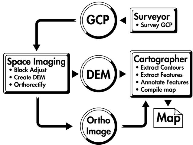
Fig. 15. Cartographic extraction from ortho images and DEM.
